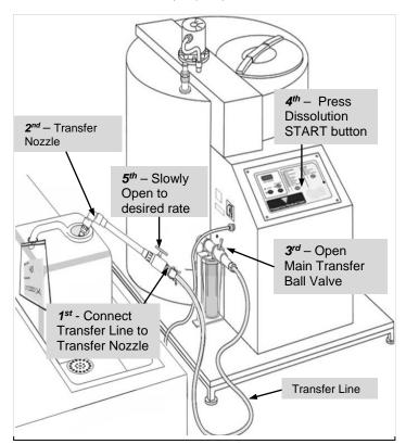
Once the manual TRANSFER Operation has been completed and the individual containers are filled, CLOSE Transfer Nozzle Valve. Press the PAUSE button.
