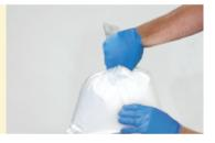
Grab the flap on the bottom of the bag and invert the bag. Insert the gathered end into the small opening in Dissolution Unit.
