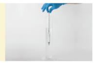
After the specific gravity value is within recommended limits, follow the instructions in your operators manual to transfer the solution to appropriate storage containers.
