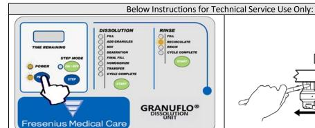
A. If the Spray Ball is stationary, push the PAUSE Button. Recirculate Light will flash. Turn Main Power Switch Off.
