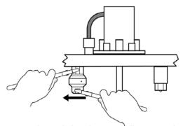
B. Remove the nut below the Spray Ball to access the sprayer.
