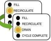
6. At the completion of the DRAIN Operation, the GranuFlo I Dissolution Unit will refill to the 25-Gallon Sensor. The Fill Indicator Light will turn on and the RINSE Operation will start.
