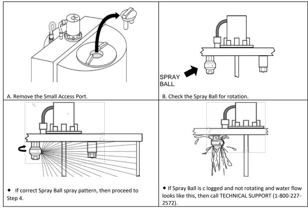
Figure 4: Spray Ball Inspection/Cleaning Instructions
