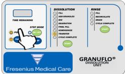
3. When the GranuFlo I Dissolution Unit is empty, the GranuFlo I Dissolution Unit will step to the CYCLE COMPLETE Operation. CLOSE the GranuFlo I Dissolution Unit's Main Transfer Ball Valve. Then Remove Transfer Nozzle and place Transfer Hose onto the Transfer Hose Holder of the Tank. Ensure you place the Transfer Nozzle in appropriate area free from dirt and other contaminates.
