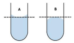
Measure the meniscus at eye level from the center of the meniscus. In the case of water and most liquids, the meniscus is concave (A). Mercury produces a convex (B) meniscus.
