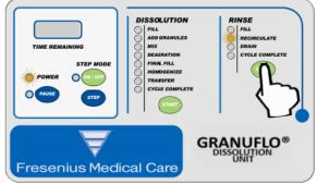
D. Press the START button on the *RINSE CYCLE* side.
