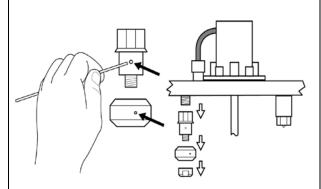
C. Clear the spray holes in both the Spray Ball and sprayer of debris and reassemble.
