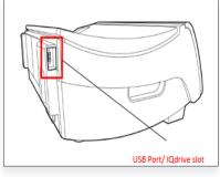
Step 1: Ensure the Kinexus Gateway is plugged into a wall outlet. Once powered on, connect the Kinexus Gateway to the cycler and insert USB drive. (Review the Kinexus Gateway's User's Guide for how to connect the Gateway to the cycler.)
