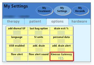
The Kinexus Gateway option automatically changes to YES when the USB drive is properly inserted and the Kinexus Gateway connection is detected by your cycler. When used with a Kinexus Gateway (shown above) and USB drive ("IQdrive™"), your cycler is capable of receiving therapy programs remotely from your clinic while you remain in the comfort of your home. Your treatment data is automatically sent to the clinic for your home therapy nurse to review.
