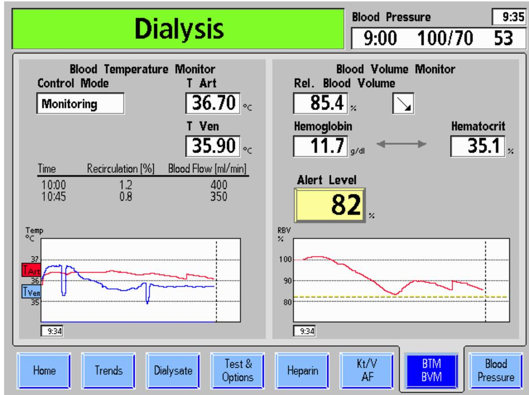
**Figure 52 – BTM and BVM Monitoring Screen**
