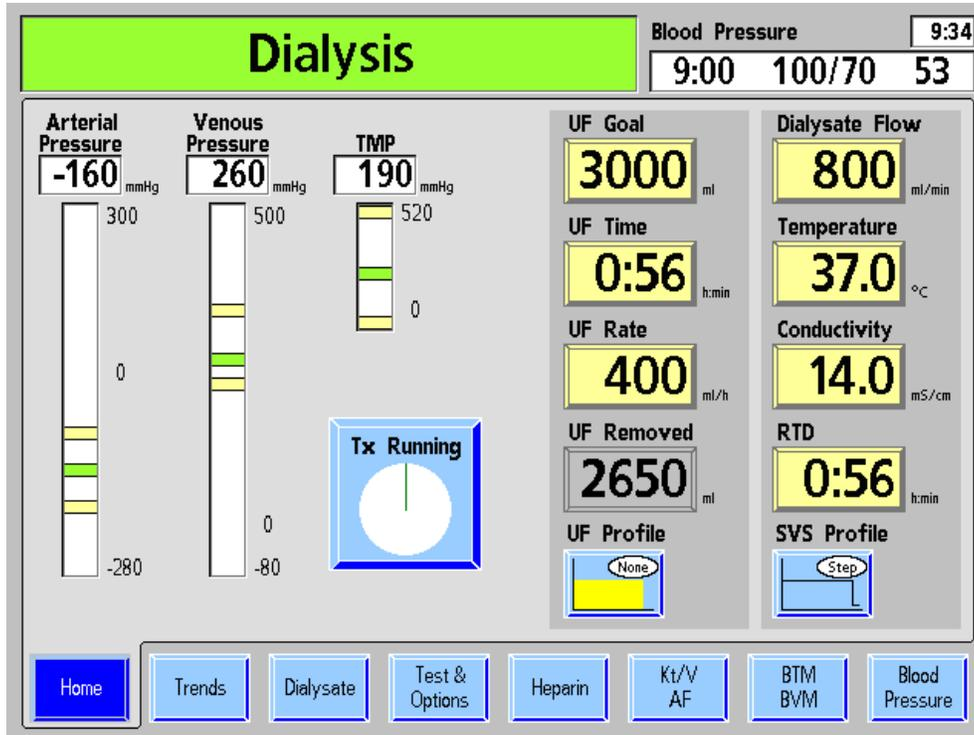
Figure 45 – Treatment Monitoring using the Home Screen
