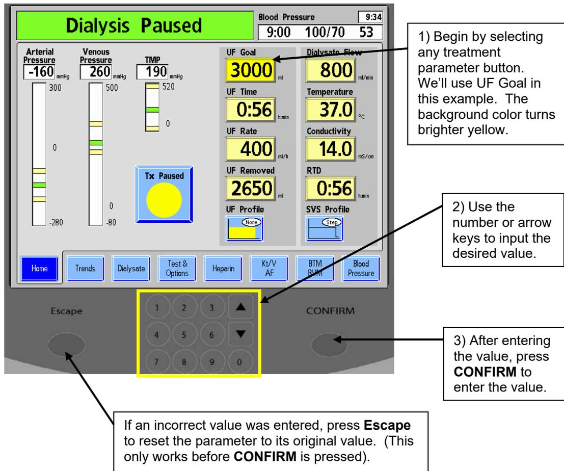
Figure 26 – Entering Parameters
