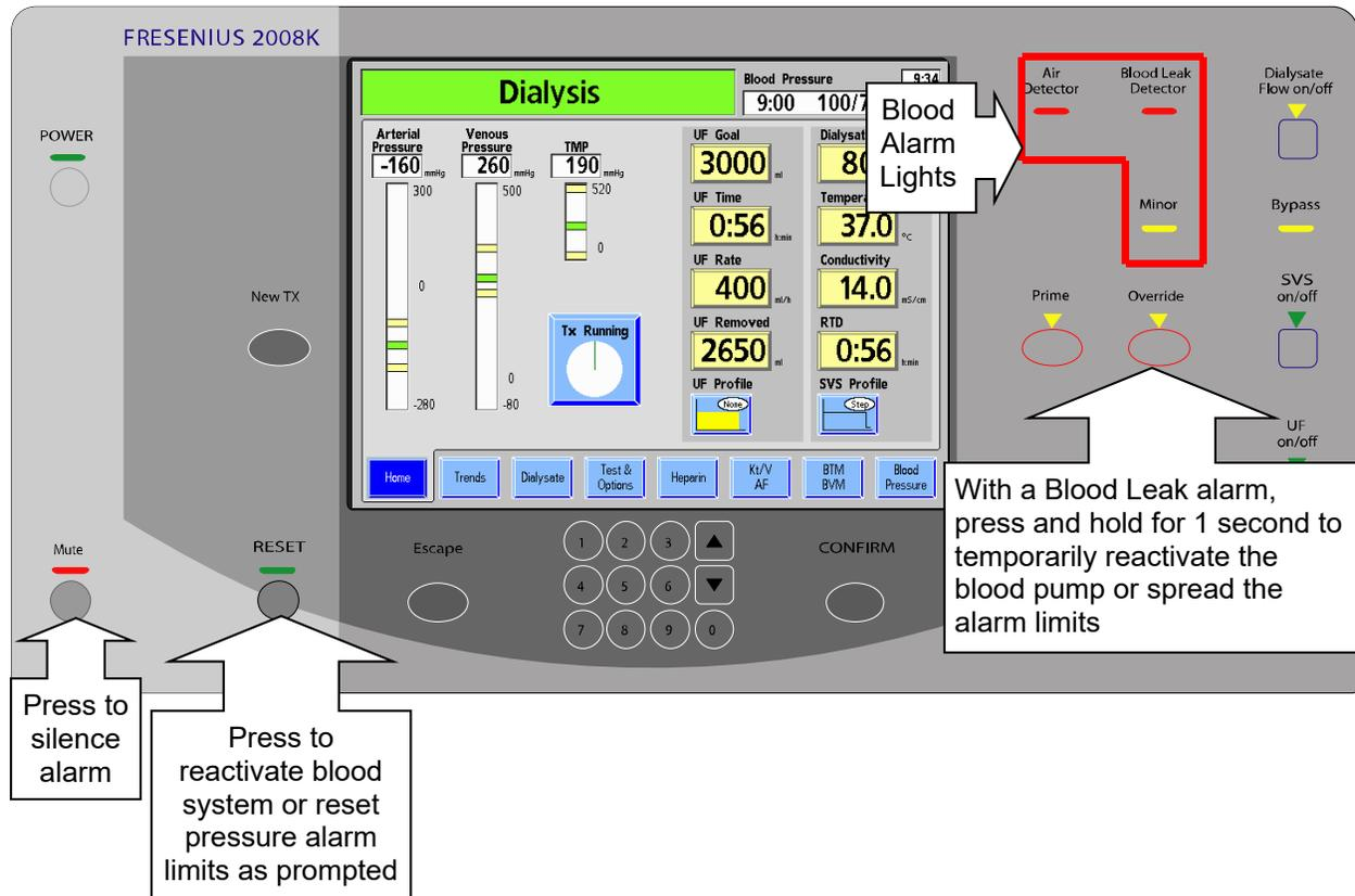
Figure 64 – Control Panel Features for Blood Alarms
