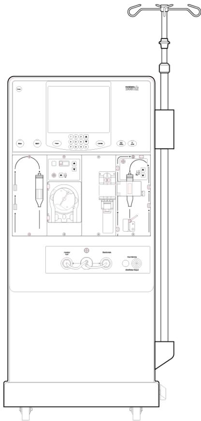
The 2008K@home hemodialysis machine is the ‘home’ version of this 2008K hemodialysis machine. The 2008K@home hemodialysis machine is designed especially for home hemodialysis patients. It features a shorter cabinet height, a simplified control panel, and on-screen guided treatment instructions for easier operation.
