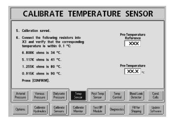
6. Insert each of the test connectors into X3 (MON-NTC) to confirm the saved calibration data. Each connector must be within 0.1°C of the Pre-Temperature data box.
