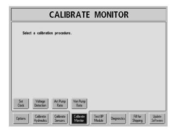
To begin a calibration, touch the appropriate calibration screen button.
