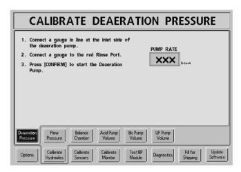
1. Connect a gauge in line at the inlet side of the deaeration pump (See Figure 1, pg. 5).
