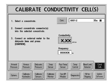
1. Identify the concentrate you will be using to calibrate the conductivity cells.
