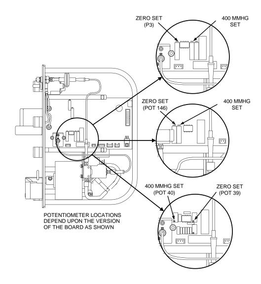
Figure 6 - Venous Pressure Display Adjustments
