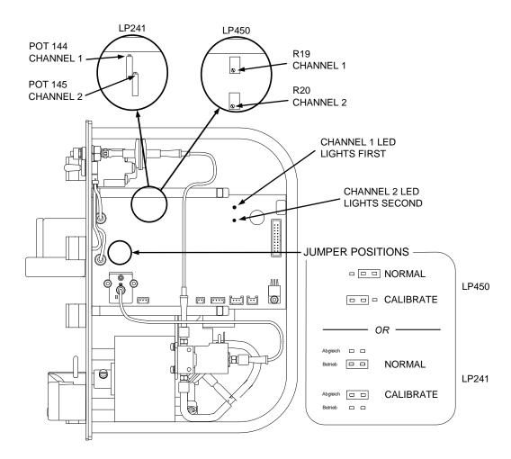
Figure 8 - Level Detector Calibration Adjustments
