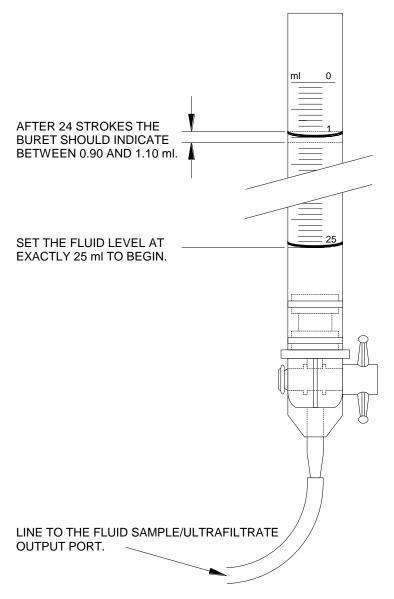
Figure 4 - UF Pump Volume Measurement
