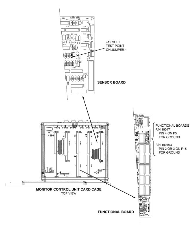
Figure 7 - +12 Volt and Ground Test Points
