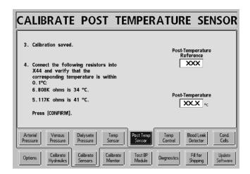
4. Insert each of the test connectors into X44 (NTC-POST) to confirm the saved calibration data. Each connector must be within 0.1°C of the Post-Temperature data box.
