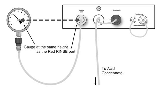
6. The loading pressure gauge in the red RINSE port will be cycling between two pressure levels. While holding the loading pressure gauge at the same height as the red RINSE port (see above), adjust pressure relief valve #65 (See Figure 1, pg. 5) for a reading between 23 and 25 psi when the gauge is reading its highest pressure level. Verify that the pressure is greater than 10 psi at the lowest level, and that it is stable within 1 psi at each level.
